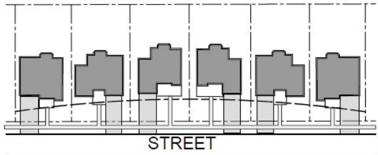
Variety of front setbacks is desirable where lot depths and block lengths permit
